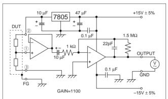
Fig. 1 Amplifier for Output Voltage Measurement
