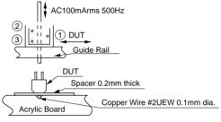
Fig. 2 Test Fixture for Output Voltage Measurement
