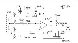
Fig. 1 Amplifier for Output Voltage Measurement
