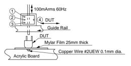
Fig. 2 Test Fixture for Output Voltage Measurement
