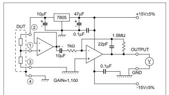
Fig. 1 Amplifier for Output Voltage Measurement
